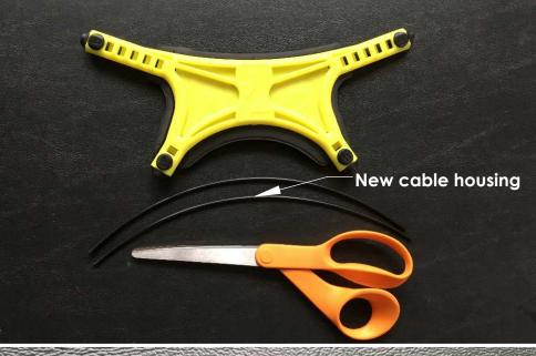
Step 27 - After cutting cable housings, open the ends with a ball point pen as shown. This will ensure the opening is round and not collapsed
