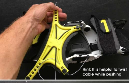
Step 37 - Push cable housing through lower leg, and pull cable and housing back through tendon back plate as shown
