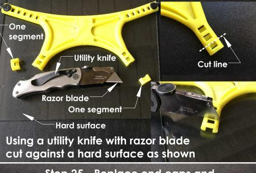
Step 25 - Replace end caps and end cap attachments as shown
