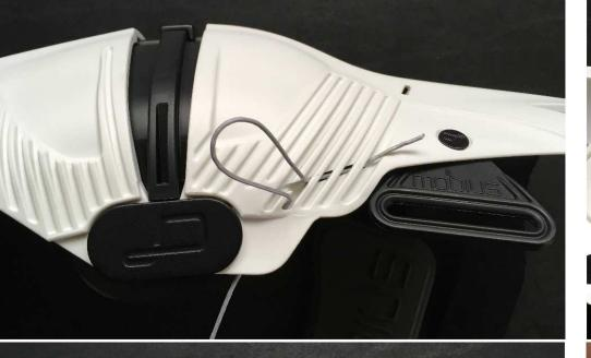
Step 13 - Pull cable to remove loop as shown
