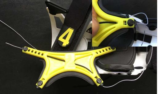
Step 34 - Push other end of cable through tendon back plate as shown
