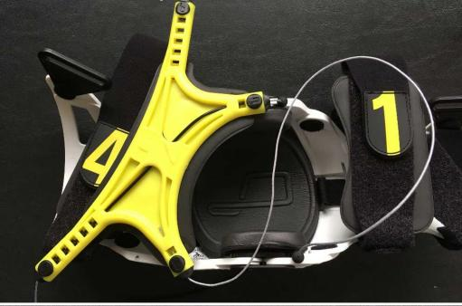
Step 35 - Push cable through cable housing as shown
