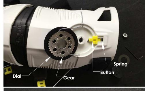
Step 7 - Loosen cable retainer screws with 1.5 mm hex wrench
