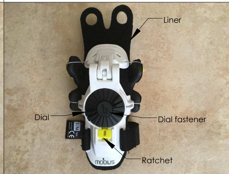
11. Assemble spring and ratchet. 12. Hold back ratchet and assemble dial ensuring cable is fully extended and not caught underneath dial. 13. Install dial fastener, washer, and screw as shown. 14. Replace liner in the desired position.
